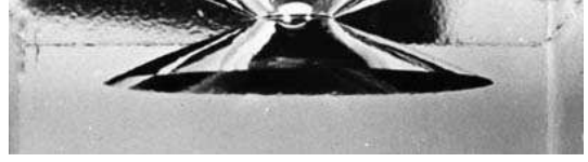
Figure 5: The hertzian cone; image taken from (30).
