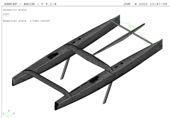
Figure 14: Finite Element Mesh of the B1 sailing race boat (Gilles Ollier Design Team, Multiplast, France)
