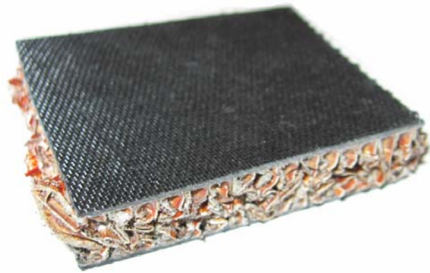
Figure 13: Sandwich specimen after crushing, Local buckling plies
