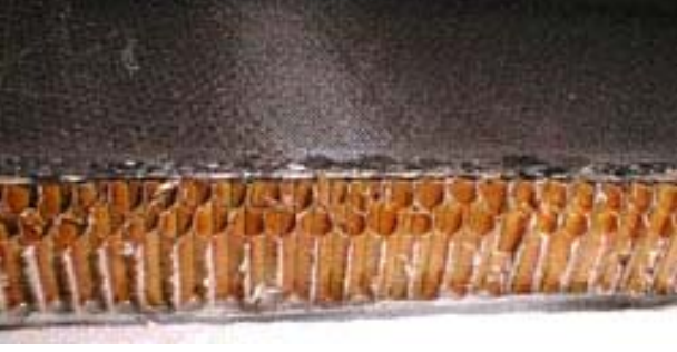
Figure 1: Sandwich, hexagonal Nomex ® core and carbon-fibre epoxy-matrix face-sheets
