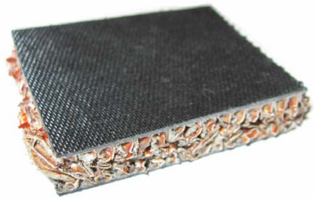
Figure 13: Sandwich specimen after crushing, Local buckling plies
