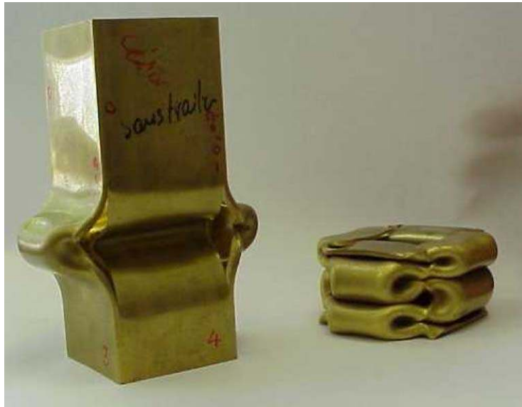
Fig. 1. Crushing mode of brass tube before (on the left) and after (on the right) heat treatment.
