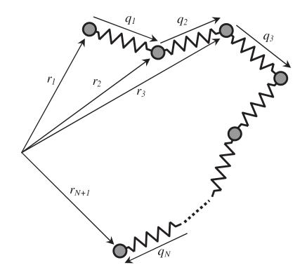
Figure 1. MBS model for polymer chain
