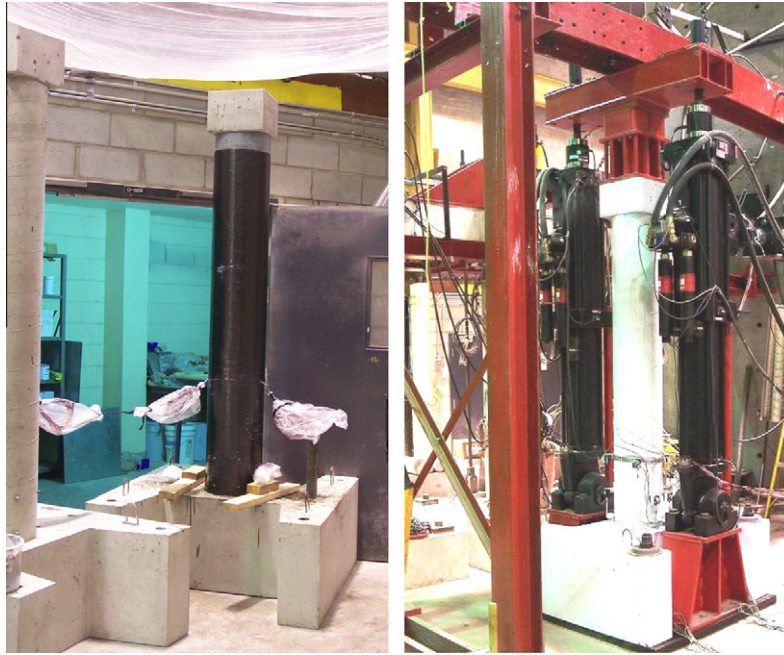
Fig. 10. RC column under cyclic loading: (left) Retrofitted and (right) unretrofitted RC column.
