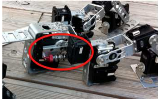
Fig. 2. Integration of Dampers in the Hip
