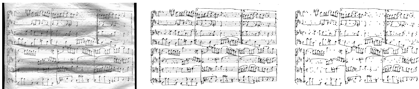
Fig. 4. From left to right: an image from TrainingSubset3, its binary version and its binary staff-less version (ground-truth)
