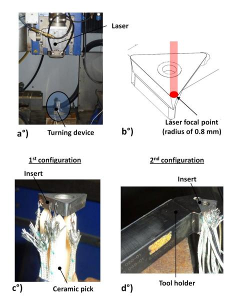
Fig. 2. Experimental device and heating configuration for the two calibration steps.
