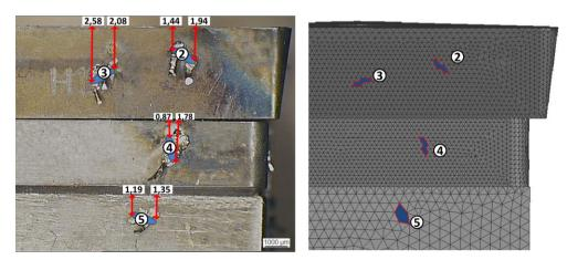
Fig. 4. Example of correspondence between thermocouple locations and set of nodes used to extract temperature results.
