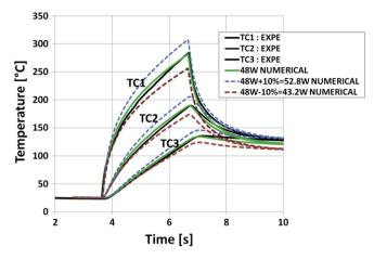
Fig. 8. Calibration of the actual laser heating power.
