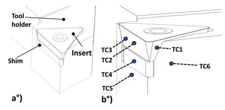
Fig. 1. Turning device and locations of thermocouples.
