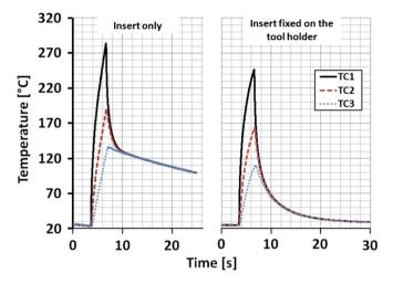
Fig. 6. Comparison of the heating and cooling curves of the insert alone and the "insert + tool-holder" set.
