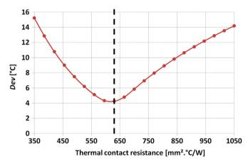
**Fig. 11.** The deviation parameter (Dev) calculated between numerical and experimental temperature results as a function of the thermal contact resistance value.
