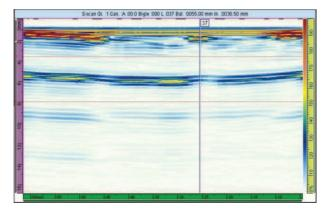
Fig. 4.6. Sectional elevation of the 2D map (S-scan).
