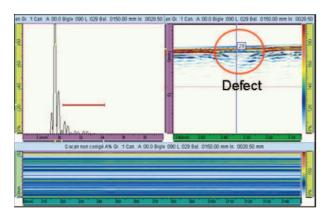
Fig. 4.10. Ultrasonic map on Specimen C.
