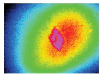
Fig. 4.7. Infrared map of the defect of Specimen B.
