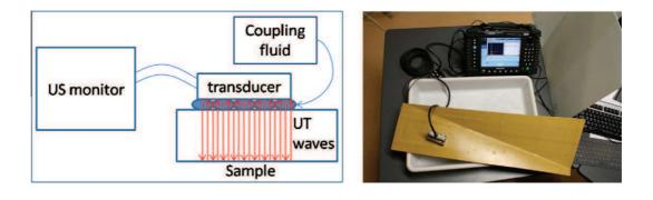
Fig. 3.1. Ultrasonic device.
