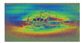
Fig. 4.3. Shearography map of Specimen A.
