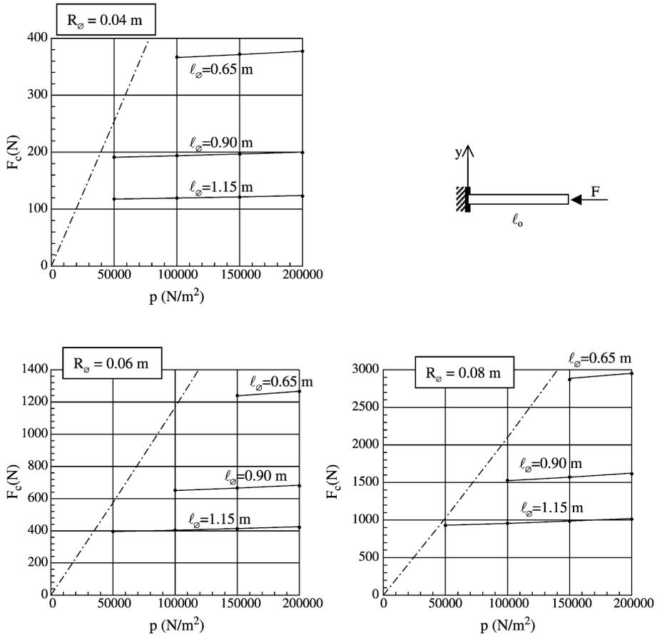
Fig. 4. Critical loads of a cantilever. (•) inflatable beam theory, ( ) membrane finite element, ( · · · ) crushing force.
