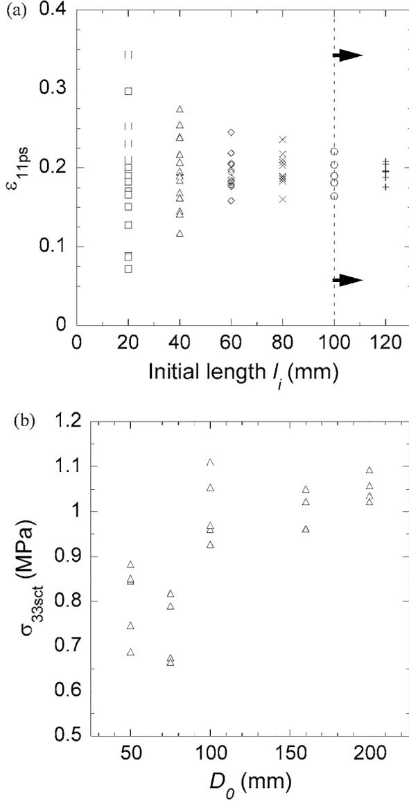
Fig. 3. (a) Plane strain compression, influence of  $l_i$  on  $\varepsilon_{33ps}$  ( $\phi = 10.8\%$ ,  $D_{33se} = 0.01 \text{ s}^{-1}$ ), and (b) simple compression, influence of  $D_0$  on stress levels ( $\phi = 14.7\%$ ,  $D_{33se} = 0.01 \text{ s}^{-1}$ ).
