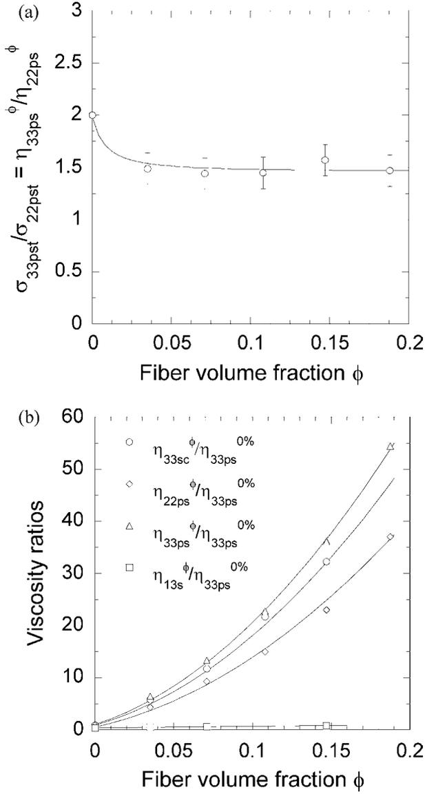
Fig. 5. Influence of the fiber content on (a) the dimensionless ratios (10)–(13) and (b) the stress ratio (14).
