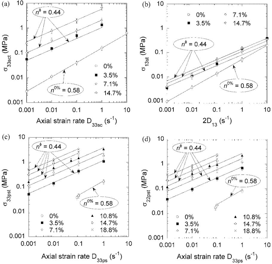
Fig. 4. Influence of the strain rate on stress levels for various fiber contents in (a) simple compression, (b) shear, (c) and (d) plane strain compression.
