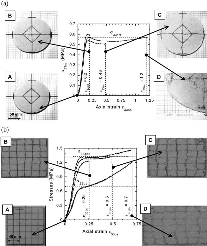
Fig. 2. Typical (a) simple compression experiments ( $\phi=14.7\%$ ,  $D_{33sc}=0.01\text{ s}^{-1}$ ) and (b) plane strain compression experiments ( $\phi=10.8\%$ ,  $D_{33ps}=0.01\text{ s}^{-1}$ ).
