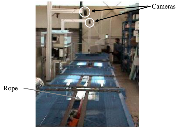
Fig. 6. 100 ton capacity test frame, test on 25 ton fiber rope.
