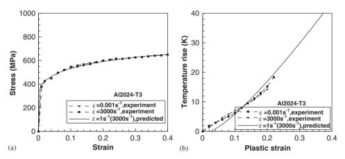
Fig. 2. (a) Stress–strain curves of Al2024-T3 at strain rate  $1 \, \text{s}^{-1}$  and  $3000 \, \text{s}^{-1}$ . (b) Adiabatic temperature rise as a function of plastic strain for Al2024-T3 at strain rate of  $1 \, \text{s}^{-1}$  and  $3000 \, \text{s}^{-1}$ . Experimental data from Hodowany et al. (2000).
