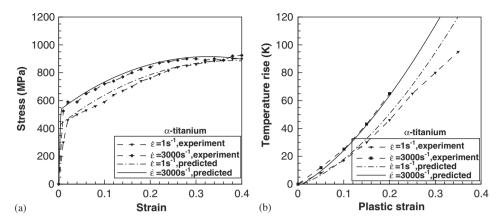
Fig. 1. (a) Stress–strain curves of  $\alpha$ -titanium at strain rate of  $1 \, \mathrm{s}^{-1}$  and  $3000 \, \mathrm{s}^{-1}$ . (b) Adiabatic temperature rise as a function of plastic strain for  $\alpha$ -titanium at strain rate of  $1 \, \mathrm{s}^{-1}$  and  $3000 \, \mathrm{s}^{-1}$ . Experimental data from Hodowany et al. (2000).
