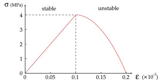
**Fig. 8.** Traction curve of the damage model.
