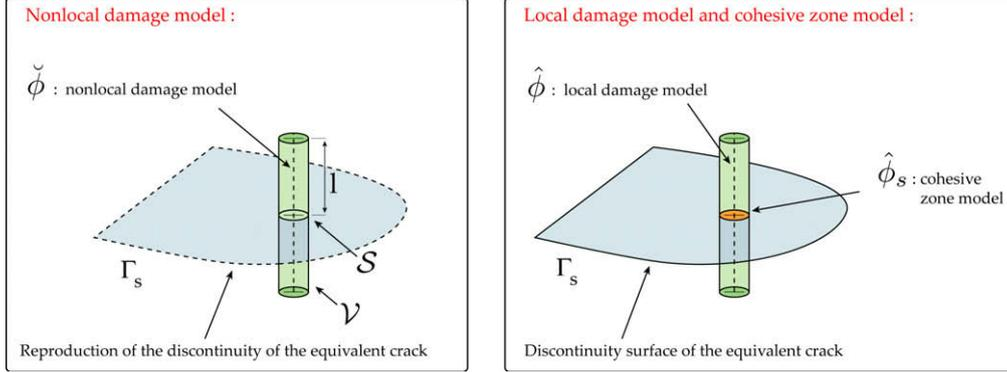
Fig. 23. Cylinders perpendicular to the discontinuity surface.
