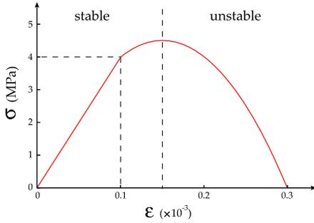
Fig. 14. Traction curve of the damage model.
