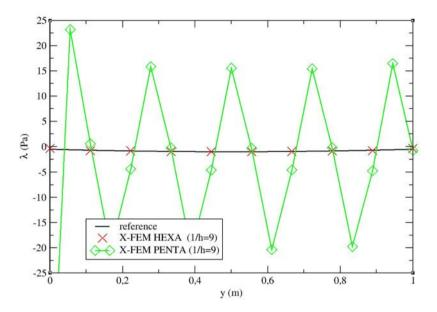
Figure 5. Contact pressure oscillations
