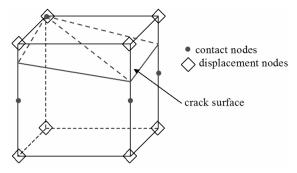
Figure 3. Example of contact sub-triangles and associated unknowns location
