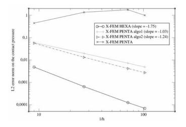
Figure 10. L2 norm error norm on the contact pressure convergence
