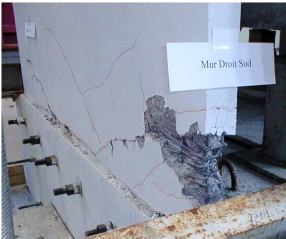
Fig. 16. CAMUS III – specimen at the end of the test (right wall).
