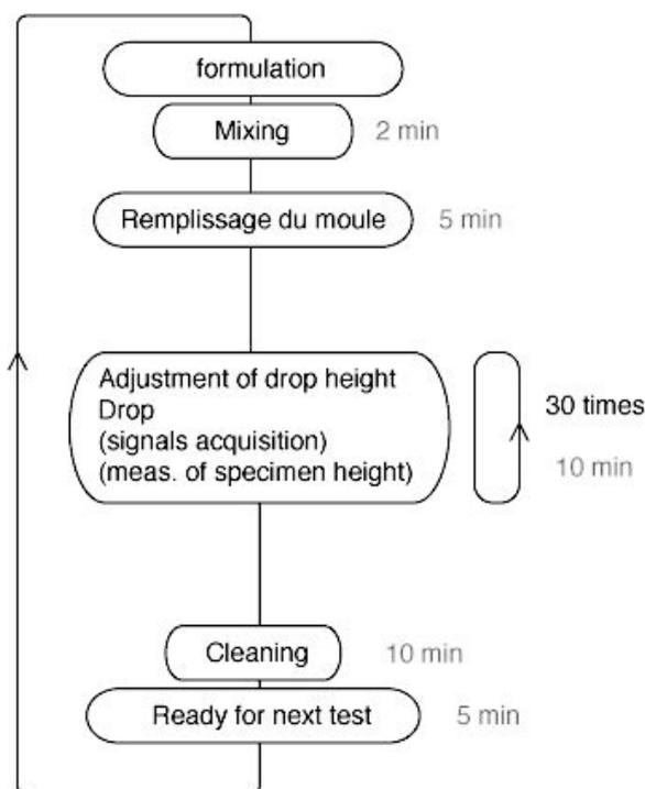
**Figure 2.** Procedure for one test.
