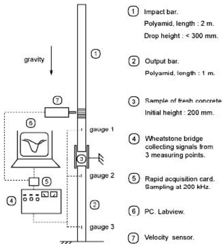
**Figure 1.** Experimental device.
