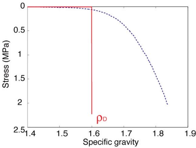
**Figure 6.** The RPPL model and a quasi-static compression test result.
