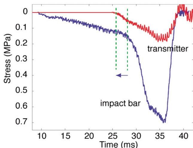
**Figure 3.** Stress measurements for the first impact.
