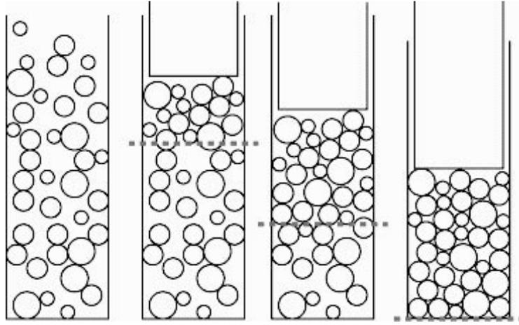
**Figure 5.** Supposed compaction process during the first impact.
