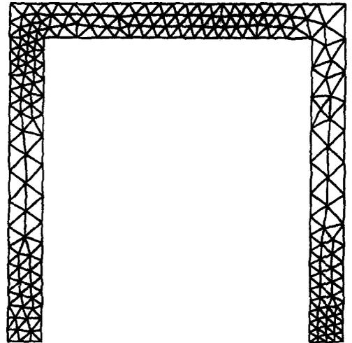
Fig. 10. The mesh: 352 three-node triangles and 235 nodes.
