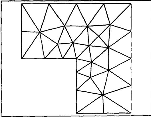
Fig. 3. The mesh: 42 six-node triangles and 103 nodes.
