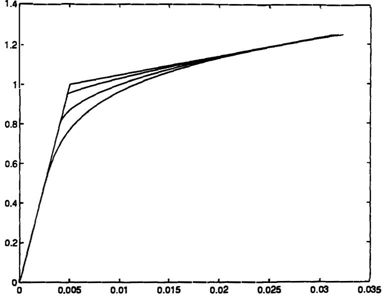
Fig. 23. Equivalent stress–strain relation for the four materials M1, M2, M3, M4 ordered from the bottom to the top.
