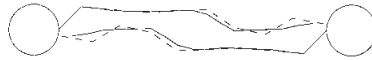
Figure 23. Crack paths for the coarse (dashed line) and fine (solid line) meshes
