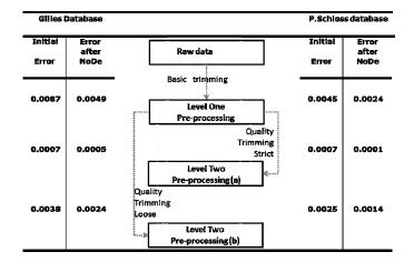
Figure 2. Flow chart showing three different pre-processing steps implemented in NoDe algorithm that aim at reducing the error rate of Gilles and P.Schloss datasets
