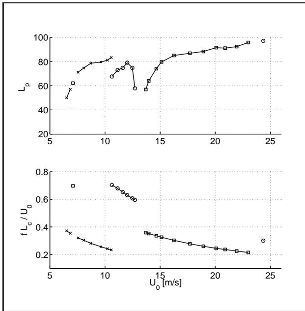
Figure 5. Sound pressure level and Strouhal number as function of  $U_0$  for 10mm cavity having a 15mm upstream section. Mode 1(240Hz, cross), mode 2(485Hz, square), mode 3(715Hz, circle), mode 4(955Hz, star).
