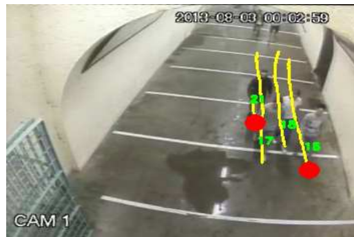
Fig. 1. Camera view and results of the automated video analysis. The yellow lines illustrate the output of the tracking algorithm. The red dots, resulting from the bobbing analysis process, indicate frames where people are estimated to start a new stride/footstep.
