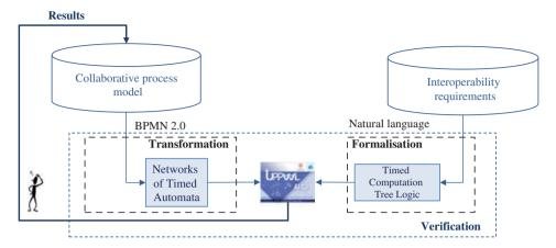
Figure 1. Verification process for interoperability requirements.
