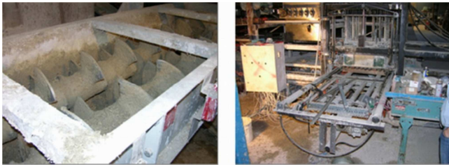
Figure 2. Precasting method (left : mixer, right : block press)
