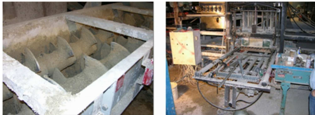
Figure 2. Precasting method (left : mixer, right : block press)
