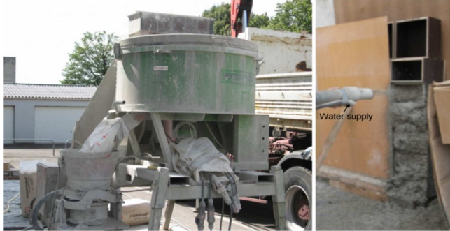
Figure 1. Spraying method (left : mixer, right : spraying hose)
