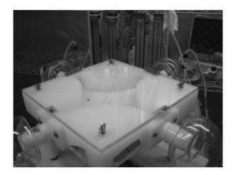
**Figure 2.** The four-way olfactometer used for SHB choice tests at the Center for Medical, Agricultural, and Veterinary Entomology (CMAVE, USDA–ARS, Gainesville, FL, USA). Filtered air is passed over bee constituents being tested and released through ports connecting the glass insect traps to the choice arena. *Photo*: Jason R. Graham.
