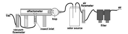
Figure 1. Lateral view of the four-way olfactometer (modified from Carroll et al., in preparation). The olfactometer is connected to an insect inlet port attached to the vacuum, drawing air from the odor source over the insect as it is released into the olfactometer. The vacuum is attached to a flowmeter (2 l/min) drawing four times the air delivered by each of the four ports (0.5 l/min), each port delivering air through air flowmeters, odor sources, and glass traps.
