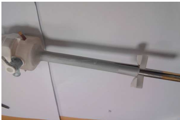
Fig. 11 Illustration of the proposed multi-view vision system (in its disposable version)
