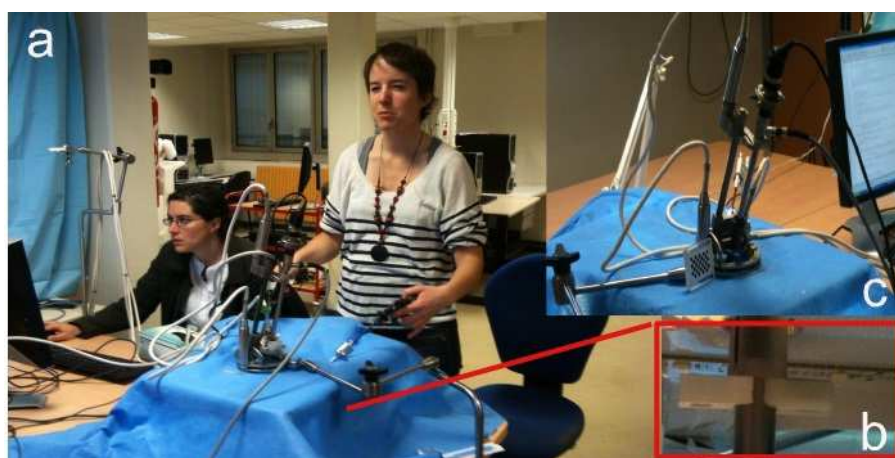
Fig. 8 Photography of the experimental set-up used to simulate the abdominal cavity and validate the different proposed materials and techniques.
