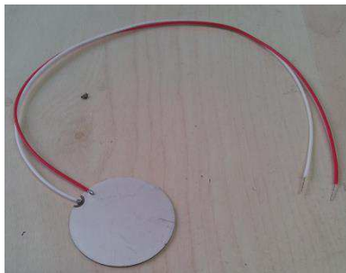
Figure 3: PZT disc from NOLIAC
