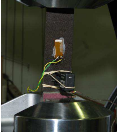
Figure 5: Tensile load of a monolithic specimen
