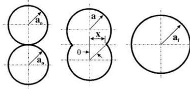
Fig. 1 Schematic sintering sequence for two cylinders, where  $a$ ,  $a_0$ ,  $a_f$ ,  $x$  and  $\theta$  are the cylinder radius, initial cylinder radius, final cylinder radius, sintering neck radius and sintering angle<sup>[3]</sup>
