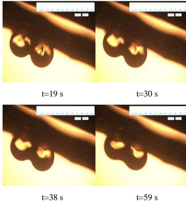
Fig. 7 Sintering sequence of ASSO fibers at 210°C
