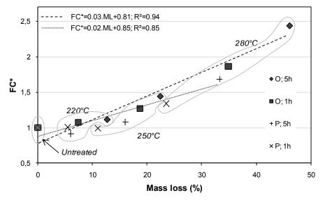
**Fig. 3.** Relative fixed carbon content (FC\*) of untreated and heat-treated wood as a function of mass loss for maritime pine (P) and pedunculate oak (O). Data grouped in each circle were subjected to the same temperature of treatment.
