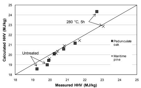
Fig. 5. HHV calculated according to Demirbas (2001) for maritime pine (P) and pedunculate oak (O) as a function of the measured HHV
