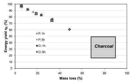
**Fig. 6.** Energy yield of maritime pine (P) and pedunculate oak (O) heat-treated under different conditions. Charcoal data comes from Schenkel et al. (1997)
