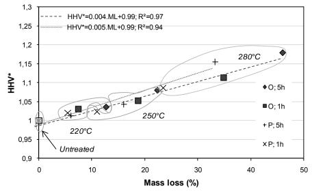
**Fig. 4.** Relative higher heating value (*HHV*\*) of untreated and heat-treated wood as a function of mass loss for maritime pine (P) and pedunculate oak (O). Data grouped in each circle were subjected to the same temperature of treatment.
