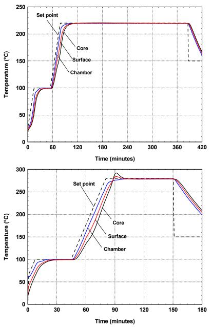
Fig. 1. The temperature evolutions for two contrasted tests (top: 220  $^{\circ}$ C – 5h and bottom: 280  $^{\circ}$ C - 1h)
