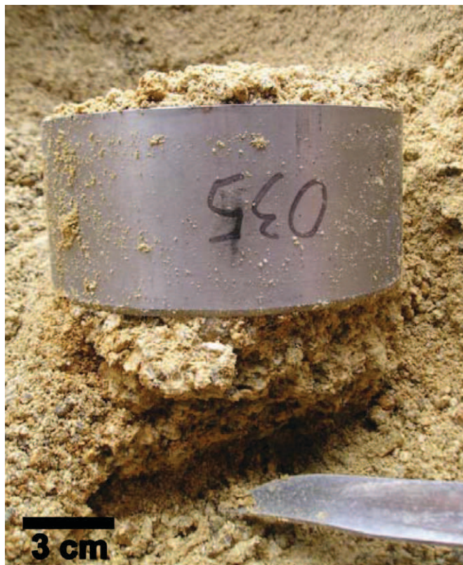
Fig. 2. A weathered granite sampler 155 cm below the soil surface with a 15-cm (inside diameter) cylinder.
