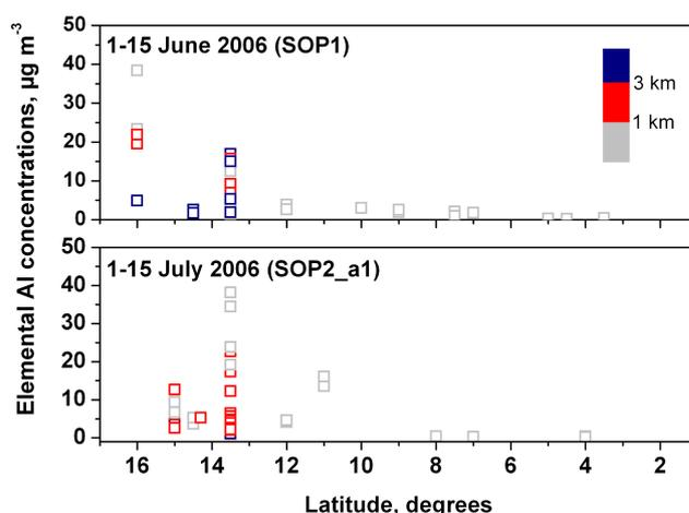
**Fig. 4.** Elemental Al concentration ( $\mu\text{g m}^{-3}$ ) as a function of latitude as determined by filter sampling during the SOP1 and SOP2\_a1 field campaigns. Data have been colour-coded according to the altitude of sampling.
