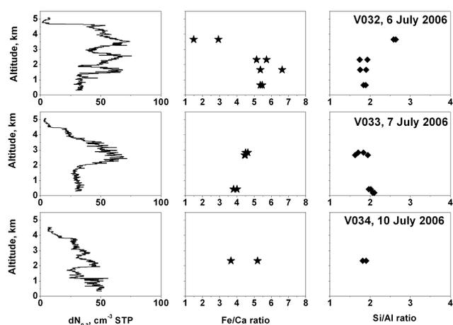
**Fig. 8.** Vertical profile of the  $dN_{0.3}$  particle number concentrations at STP conditions (left panel), Fe/Ca elemental ratio (central panel) and Si/Al elemental ratio (right panel) for the Sahelian dust uplift and transport episodes observed north of Banizoumbou on 6 July (flight V032, upper row), 7 July (flight V033, mid-row) and 10 July (flight V034, lower row) during a Sahelian uplift and transport event.
