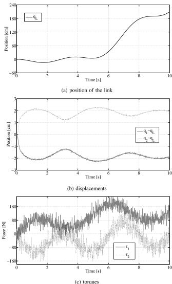
Fig. 4. Noisy signals used for the simulations.
