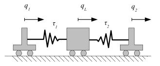
Fig. 7. Translational model of a VSA, as the one used in the experimental setup.
