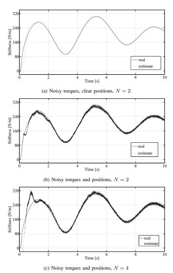
Fig. 5. Reconstruction of the stiffness in simulation.
