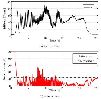
Fig. 9. Results of experiment: performance of the observer tracking the stiffness of an Agonist-Antagonist VSA.
