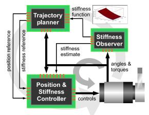
Fig. 2. A possible control system for a Variable Stiffness Actuator, organized in two layers: On the lowest layer a position and stiffness controller tracks the references generated by the higher level trajectory planner. Both control loops rely on knowledge on the stiffness of the actuator: the instantaneous value of the stiffness is used to close the inner loop, while the shape of the stiffness function is used by the trajectory planning algorithm.
