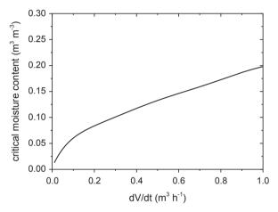
Fig. 8. Critical moisture content as a function of evaporation rate as predicted by Eq. (2).
