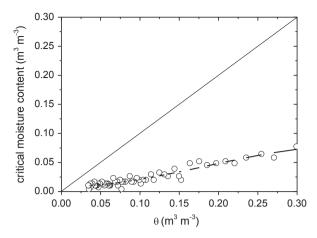
**Fig. 9.** Critical moisture content as a function of water content in the material for salt satured fired-clay brick with 0% RH as predicted by Eq. (5).
