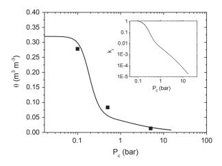
**Fig. 7.** Capillary pressure curve for fired-clay brick material. The filled symbols are experimental data (Pel et al., 2010). The solid line is computed using Eq. (3). The insert shows the relative permeability computed using Mualem's model (Eq. (4)).
