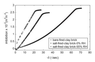
**Fig. 6.** The measured imbibition of decane in the salt-free fired-clay brick and in firedclay bricks saturated with 3 m NaCl solution dried at different relative humidity conditions.
