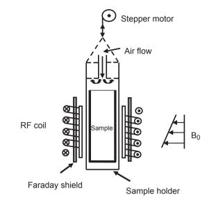
**Fig. 1.** NMR set-up for the drying experiments with cylindrical samples. The Teflon holder with the saturated sample is moved in the vertical direction by means of a stepper motor. The signal from H or Na nuclei at resonance is received by the RF coil.
