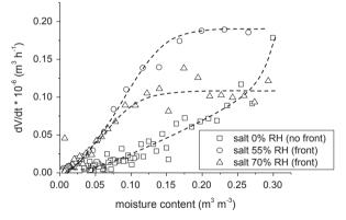
**Fig. 4.** The rate of water volume change (dV/dt) as a function of moisture content  $(m^3 m^{-3})$  for salt saturated bricks dried at different relative humidity conditions. The dashed lines are a guide to the eve.
