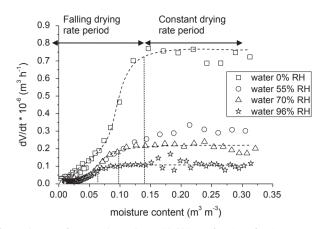
**Fig. 3.** The rate of water volume change (dV/dt) as a function of moisture content  $(m^3 m^{-3})$  for water saturated fired-clay bricks dried at different relative humidity conditions. The dashed lines are guide to the eye.
