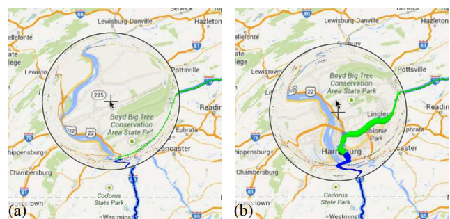
Figure 1: Following an itinerary. (a) Conventional lens: the user overshoots at a right turn in Harrisburg; losing the route that falls in the distorted region. (b) RouteLens: the route’s attraction compensates the overshoot; the lens remains closer to the route, which remains in focus.
