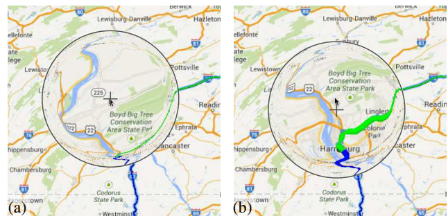
Figure 1: Following an itinerary. (a) Conventional lens: the user overshoots at a right turn in Harrisburg; losing the route that falls in the distorted region. (b) RouteLens: the route’s attraction compensates the overshoot; the lens remains closer to the route, which remains in focus.
