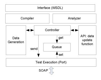
Figure 6. Online testing framework architecture
