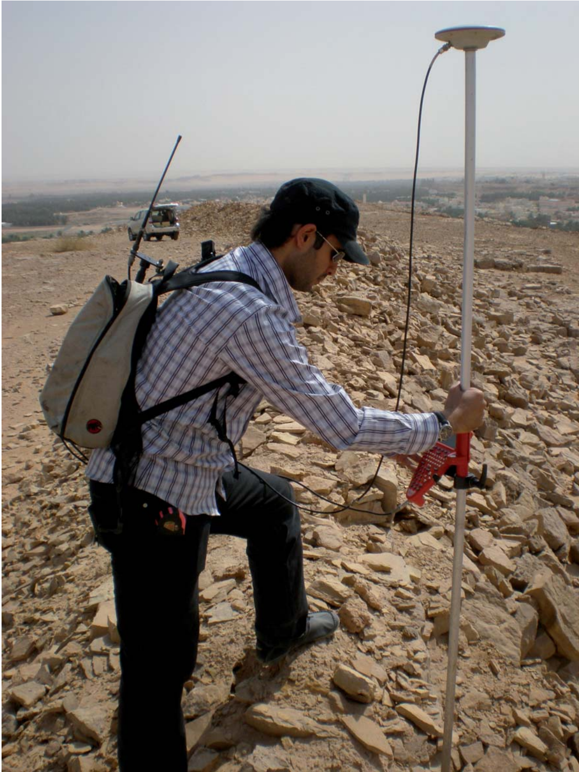
Fig. 6. Thâmir 'A. al-Mâlikî (SCTA) surveying the western enclosure wall with a differential GPS
