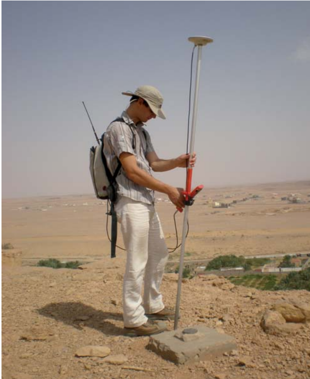
Fig. 1. Quentin Morel using a differential GPS
