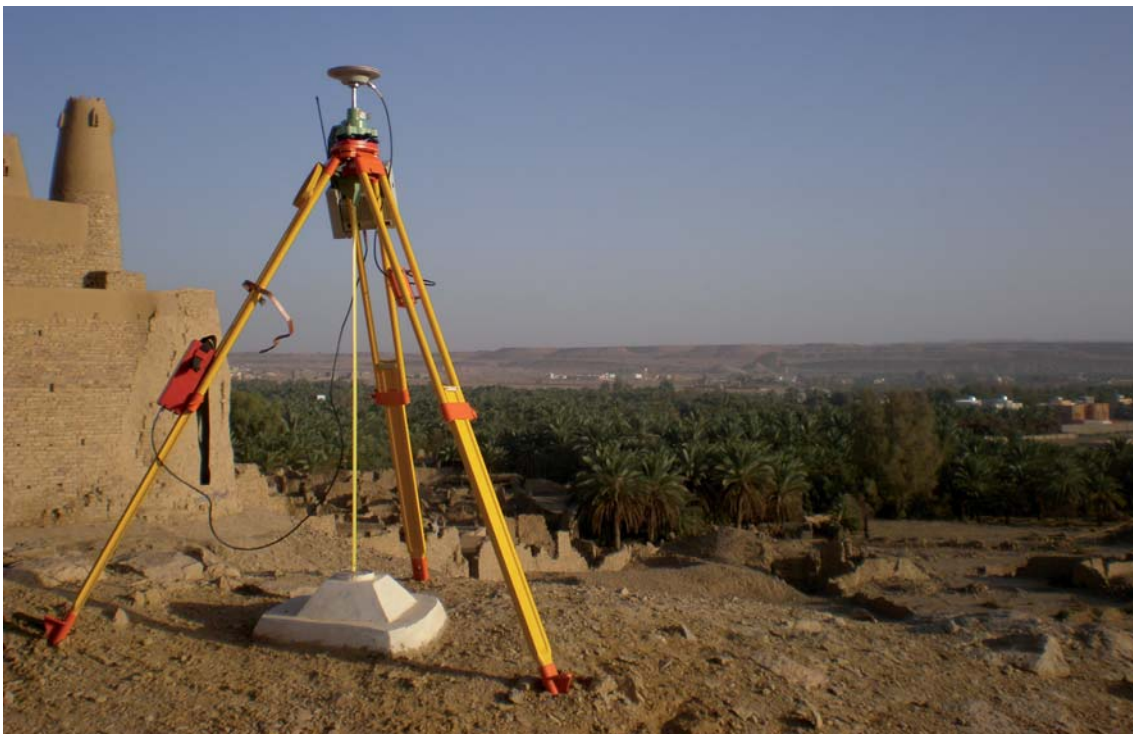
Fig. 2. Differential GPS pivot
