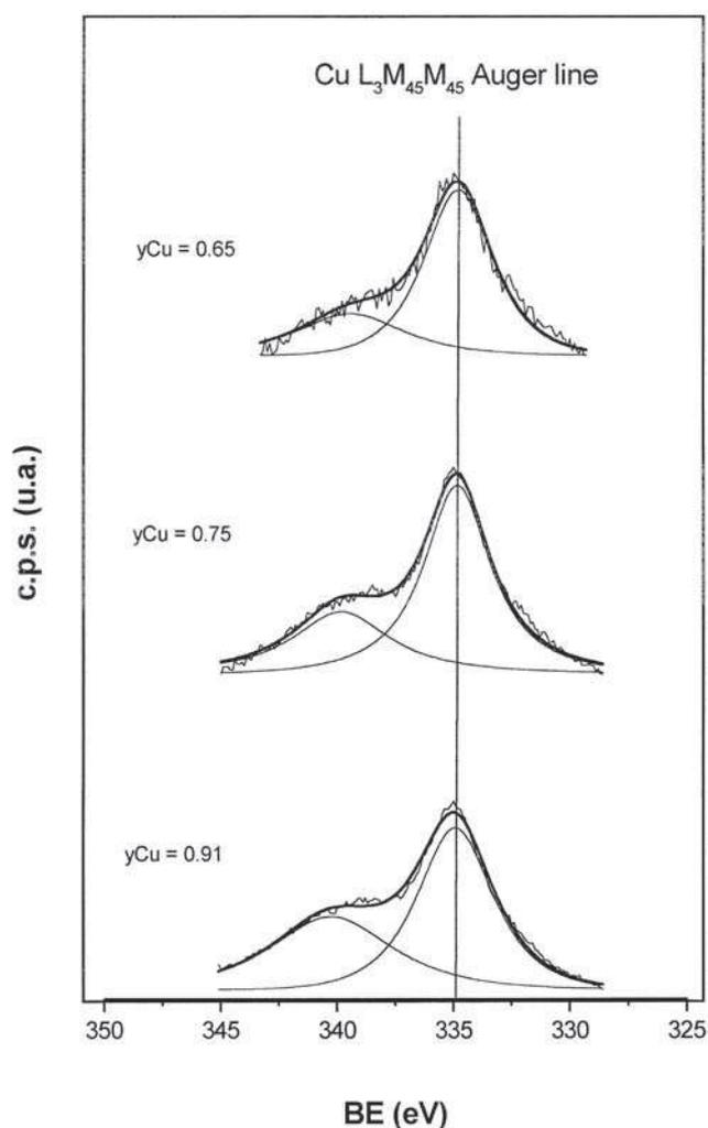
Fig. 4. Cu L<sub>3</sub>M<sub>45</sub>M<sub>45</sub> Auger transition for Ni<sub>0.70</sub>Cu<sub>y</sub>Mn<sub>2.3-y</sub>□<sub>3δ/4</sub>O<sub>4+δ</sub> with y<sub>Cu</sub> = 0.65, 0.75 and 0.91.
