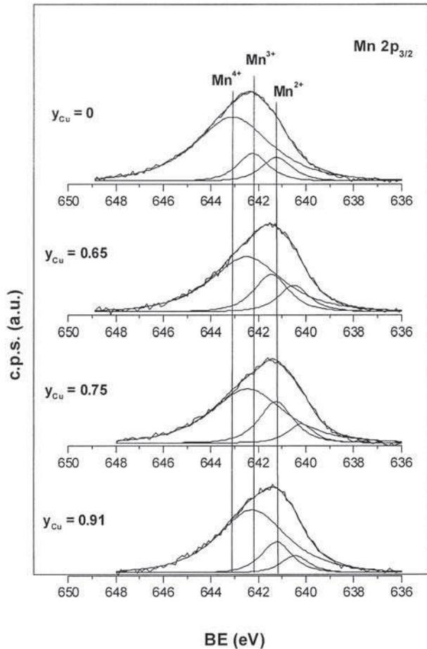
Fig. 5. Mn $2p_{3/2}$  core-level spectra for  $\text{Ni}_{0.70}\text{Cu}_y\text{Mn}_{2.3-y}\square_{3\delta/4}\text{O}_{4+\delta}$  with  $y_{\text{Cu}} = 0, 0.65, 0.75$  and  $0.91$ .
