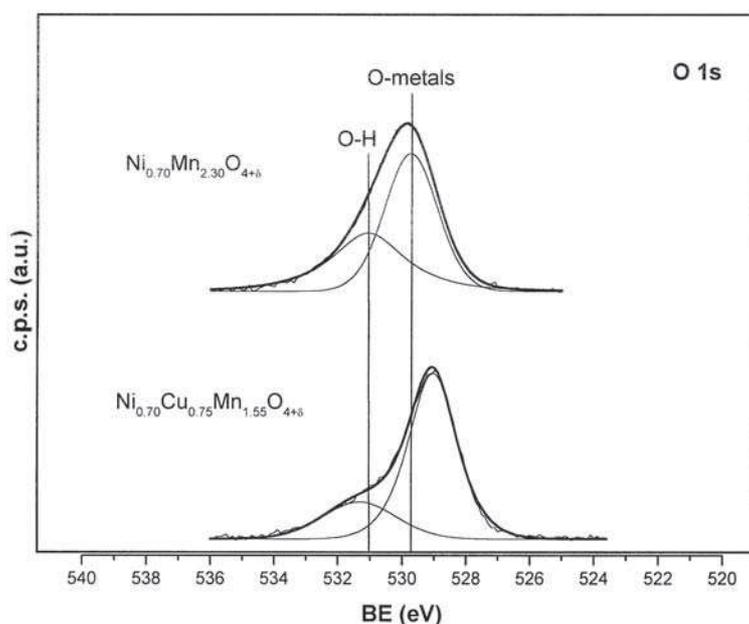
Fig. 2. O 1s core-level spectra of the O 1s region for Ni<sub>0.70</sub>Mn<sub>2.30</sub>O<sub>4.70</sub> and Ni<sub>0.70</sub>Cu<sub>0.75</sub>Mn<sub>1.55</sub>O<sub>4.25</sub>.
