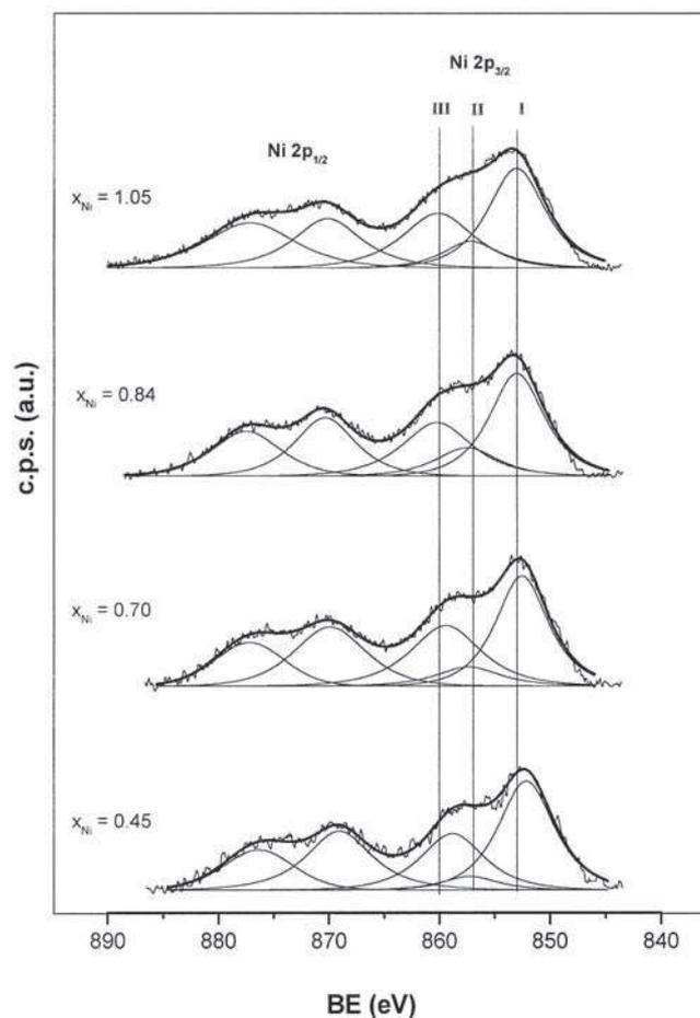
Fig. 1. Ni 2p core-level spectra for Ni $_x$ Mn $_{3-x}$ □ $_{3\delta/4}$ O $_{4+\delta}$  with  $x_{Ni}=0.45, 0.70, 0.84$  and  $1.05$ .
