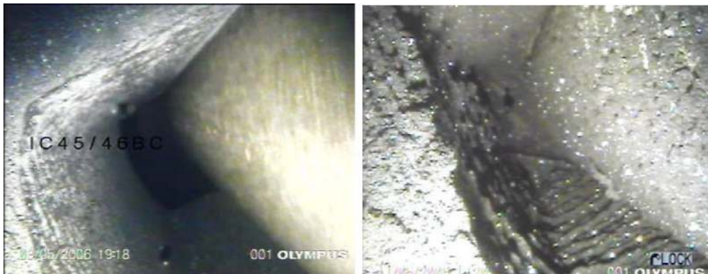
Fig. 3. Photo of Tube Support Plate flow blockage: top view of a “clean” flow hole on the left side and an entirely blocked flow hole on the right side (tube on the right side).
