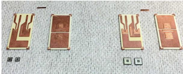
Figure 5: Two sets of parts (one for the  $2.4 \times 2.4 \text{ mm}^2$  JFET dies, one for the  $4 \times 4 \text{ mm}^2$  JFET dies) before assembly. A set comprises two ceramic tiles, two JFETs and one spacer.
