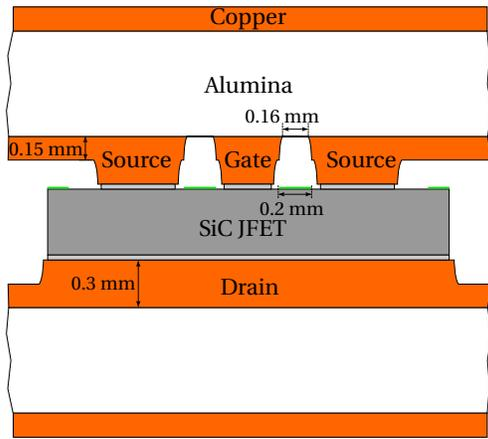
Figure 2: Up-to-scale cross section of the sandwich module around the SiC die (here a  $2.4 \times 2.4 \text{ mm}^2$  die) showing the relative thicknesses and spacing between the copper tracks. The alumina thickness is  $0.635 \text{ mm}$ , and that of the sintered-silver layer  $\approx 0.025 \text{ mm}$ .
