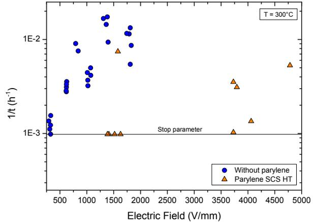
Figure 4: Time before a short circuit appears between the electrodes of a test sample as a result of silver migration, for an ambient temperature of  $300 \text{ }^\circ\text{C}$ , depending on the electric field applied, and for two sets of samples: unprotected (blue dots), and coated with a  $20 \mu\text{m}$  layer of parylene HT (yellow triangles).
