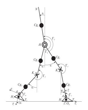
Fig. 1. Biped robot with rolling joint knees
