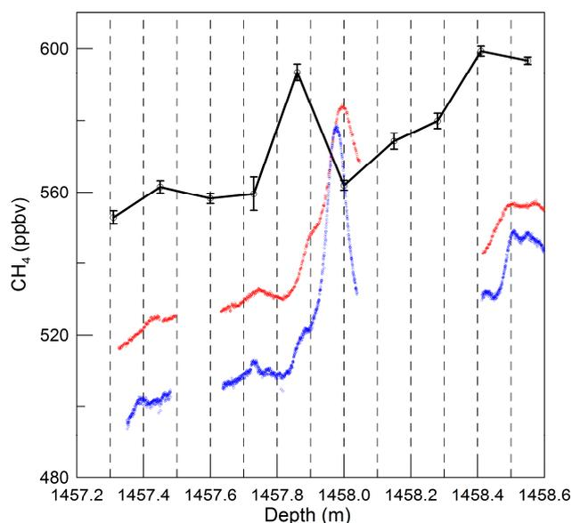
**Fig. 4.** Zoom over 1.4 m of the  $\text{CH}_4$  profiles, located in the Bølling/Allerød – Younger Dryas transition. Discrete OSU measurements (black circles with error bars) show a small depth shift with the WS-CRDS (red dots) and OF-CEAS (blue dots) uncorrected raw data on their respective depth scales.
