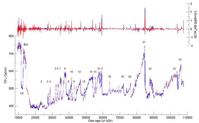
**Fig. 9.** Calibrated laser spectroscopic CH<sub>4</sub> profiles (blue: OF-CEAS; red: WS-CRDS) from 107.7 to 9.5 ka b2k (GICC05modelext time scale) and associated rates of CH<sub>4</sub> change (same colour code). Numbers correspond to Greenland interstadials (GIS, or Dansgaard–Oeschger events). YD stands for Younger Dryas, and B/A for Bølling/Allerød.
