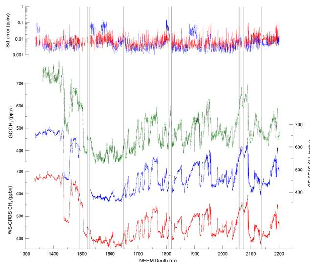
**Fig. 5.** Lower graphs: WS-CRDS (red), OF-CEAS (blue) and GC (green) data sets in the depth domain before applying mixing ratio corrections. Dashed black lines fill the gaps in each data set. The OF-CEAS and WS-CRDS data are averaged on 20 cm increments. Vertical grey lines correspond to depths where a change in the analytical setup took place, which affected the results (Table 1). Upper graph: standard error of the mean for each 20 cm increment (blue: OF-CEAS; red: WS-CRDS).
