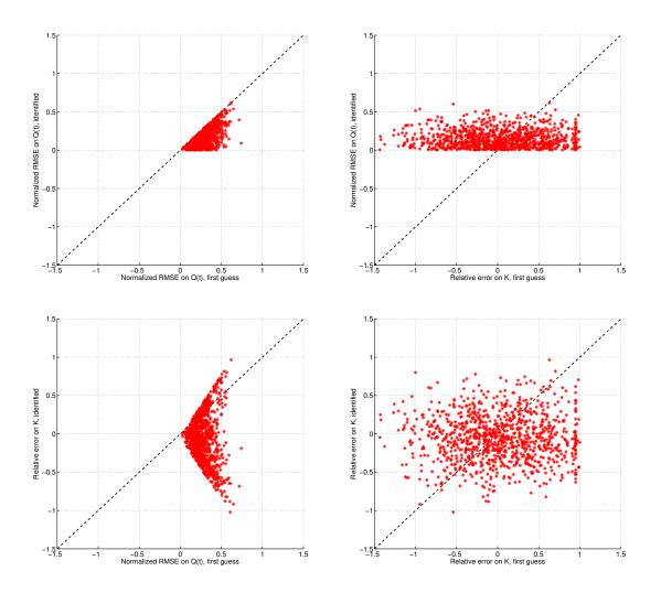
Figure 11: Sensitivity of discharge and roughness identification to first guess. Results are represented in the different planes  $(Err_K, Err_{K_b})$ ,  $(Err_Q, Err_{Q_b})$ ,  $(Err_K, Err_{Q_b})$ ,  $(Err_Q, Err_{K_b})$ , for a sample of 1000 sets of random gaussian first guesses. Water surface observations are used with expected SWOT like errors.  $x_{situ} = 12$  km. The error on K can be positive or negative. Flow features are summed up in Table 1 and Figure 4.
