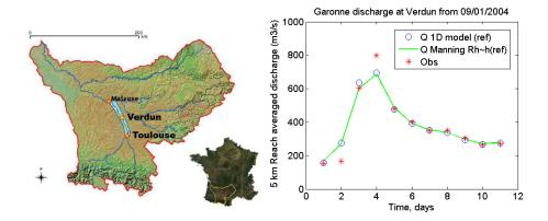
Figure 5: (left) The Garonne River study area between Toulouse-Malause, and the location of the validation gauge of Verdun sur Garonne. (Right) Comparison of observed discharge at Verdun sur Garonne with reach averaged Manning equation and 1D reference SW model for the period of interest.
