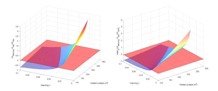
Figure 2: Forward problem, response surface of Gauckler–Manning–Strickler equation (colored surface) and best discharge estimation (transparent red plane) for (left) one and (right) three permanent states of a reach of the Garonne river test case
