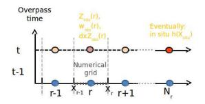
Figure 3: Forward problem grid: numerical grid within a hydraulic grid consisting in a discretization of a river into reaches (r) from SWOT observation grid. Reach boundaries defined by in-situ cross section measurements.
