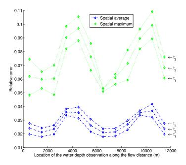
Figure 9: Mean  $(\|.\|_1)$  and maximum  $(\|.\|_{\infty})$  spatial errors on bathymetry identification (low Froude inverse model, observations=backwater curve) in function of the location of the in-situ water depth measurement, "perfect observations". Flow features are summed up in Table 1 and Figure 4.
