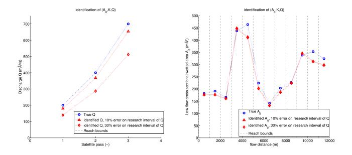
Figure 6: Results obtained while performing the triplet  $(A_0, K, Q)$  identification : (left) the discharge Q, (right) the base-flow cross sectional area  $A_0$ , and the roughness  $K = 20.1 \ m^{1/3} \cdot s^{-1}$  (the truth being  $K_t = 20 \ m^{1/3} \cdot s^{-1}$ ). Observations with SWOT like errors. Flow features are summed up in Table 1 and Figure 4.
