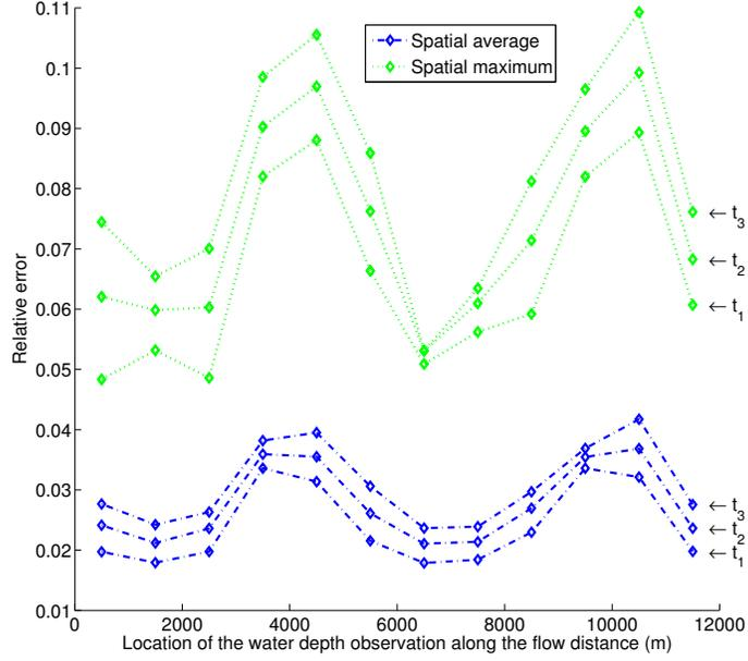
Figure 9: Mean ( $\|\cdot\|_1$ ) and maximum ( $\|\cdot\|_\infty$ ) spatial errors on bathymetry identification (low Froude inverse model, observations=backwater curve) in function of the location of the in-situ water depth measurement, “perfect observations”. Flow features are summed up in Table 1 and Figure 4.
