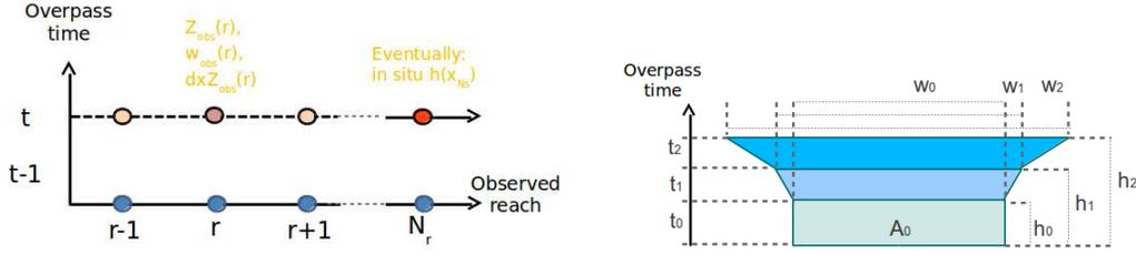
Figure 1: Inverse model discretization. (left) The spatial grid of observations is imposed by the instruments. The hydraulic sections-reaches ( $r$ ) grid fits the observation grid. (right) Section view. Time overpasses are ordered by increasing flow height. The lower wetted-section  $A_0$  is not measured.
