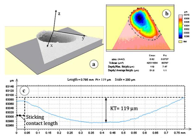
Fig. 6. (a) 3D crater wear topography (Vc = 500 m/min, feed = 0.1 mm/rev et doc = 1.1 mm), (b) determination of crater wear volume (VKT,  $\mu m^3$ ), (c) profile of crater perpendicular to cutting edge, determination of KT ( $\mu m$ ) in plane (x, z).
