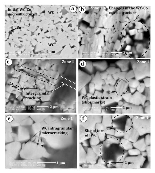
$\textbf{Fig. 9.} \ (a) \ Initial \ micrograph \ of \ WC-6Co, \ (b)-(f) \ crater \ wear \ SEM \ micrographs \ for \ detail \ observations \ zone \ 1 in \ Fig. \ 8b.$
