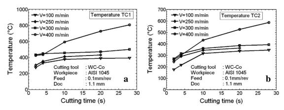
**Fig. 3.** Cutting tool temperature evolution vs. time for four cutting speeds: (a) - TC1; (b) - TC2.
