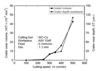
$\textbf{Fig. 7.} \ \textbf{Evolution of crater wear volume of and crater wear depth vs. cutting speed.}$
