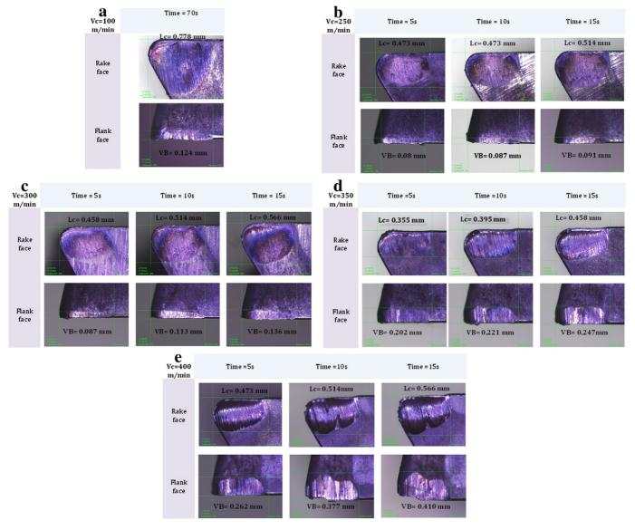
Fig. 5. Evolution of crater wear and flank wear of the cutting tools at macroscopic observations for different cutting speed, (magnification 216×).
