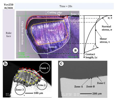
**Fig. 8.** (a) Evolution of normal and shear stress at tool–chip contact zones (feed  $= 0.1 \, \text{mm/rev}$ , doc  $= 1.1 \, \text{mm}$ ), (b) three zones define for wear analysis and (c) SEM micrographs of crater wear of the cutting tool cross-section, perpendicular to the cutting edge (Vc  $= 400 \, \text{m/min}$ , feed  $= 0.1 \, \text{mm/rev}$ , doc  $= 1.1 \, \text{mm}$ ).
