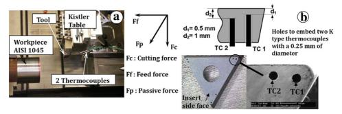
Fig. 1. (a) Experimental setup for machining tests, (b) detail of cutting tool insert.
