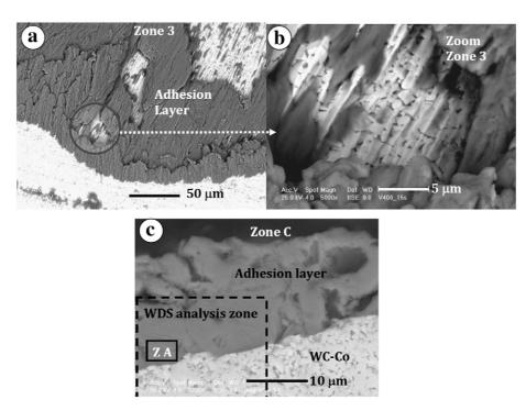
Fig. 11. Crater wear SEM micrographs for detail observations: (a) and (b) zone 3 in Fig. 8b, (c) zone C in Fig. 8c.
