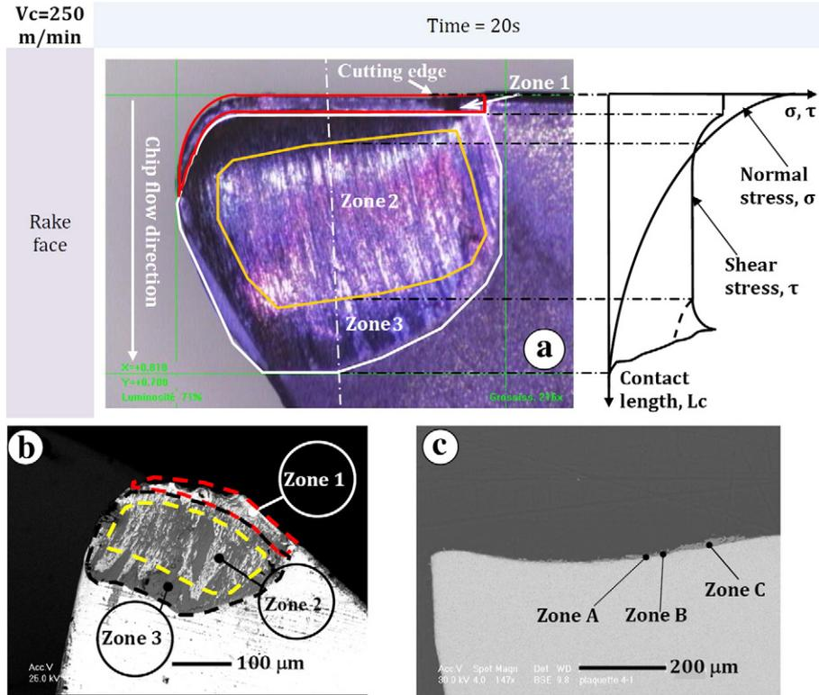
**Fig. 8.** (a) Evolution of normal and shear stress at tool–chip contact zones (feed = 0.1 mm/rev, doc = 1.1 mm), (b) three zones define for wear analysis and (c) SEM micrographs of crater wear of the cutting tool cross-section, perpendicular to the cutting edge ( $V_c = 400$  m/min, feed = 0.1 mm/rev, doc = 1.1 mm).
