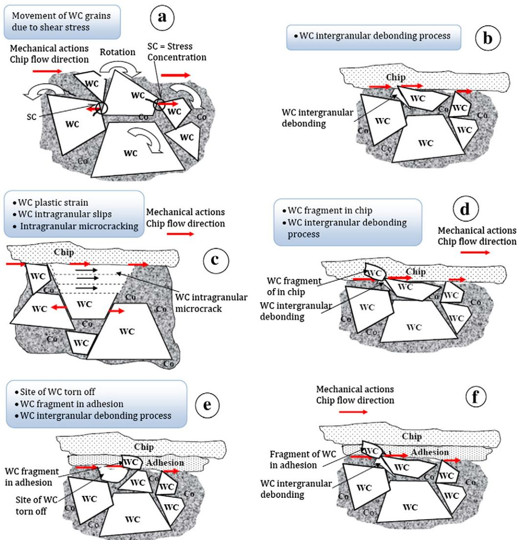
**Fig. 14.** Wear micromechanisms phenomena identified in crater.
