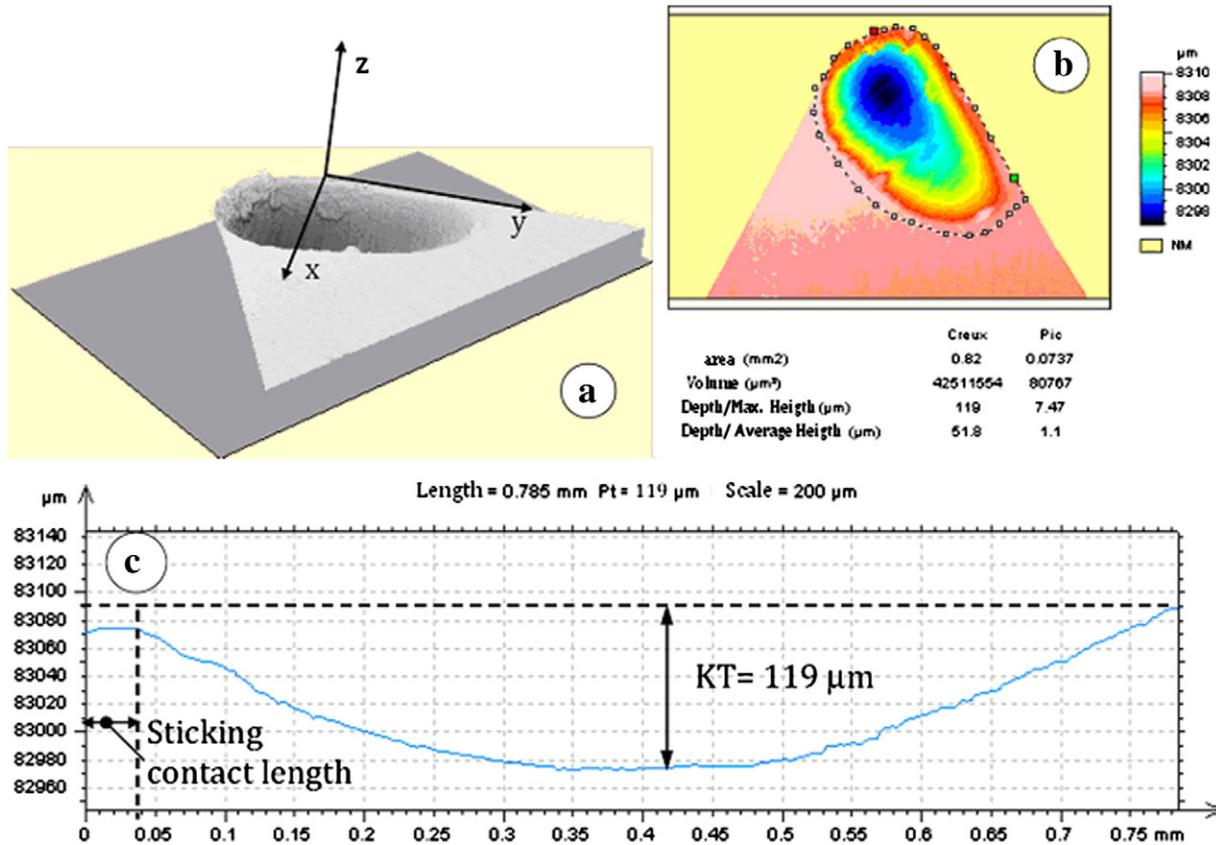
Fig. 6. (a) 3D crater wear topography ( $V_c = 500$  m/min, feed = 0,1 mm/rev et doc = 1,1 mm), (b) determination of crater wear volume ( $V_{KT}, \mu\text{m}^3$ ), (c) profile of crater perpendicular to cutting edge, determination of  $KT$  ( $\mu\text{m}$ ) in plane  $(x, z)$ .
