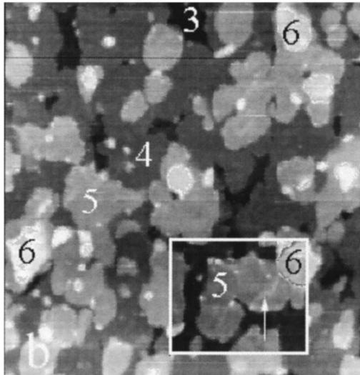
FIG. 6.  $1260 \times 1330$ -Å STM view of a 5-ML-thick Co layer grown at  $-1.6$  V. The contrast was enhanced in the square boxes to show structural defects. This image must be compared to the last frame of Fig. 5. Figures  $N$  inside images are the local number of Co atomic monolayers.
