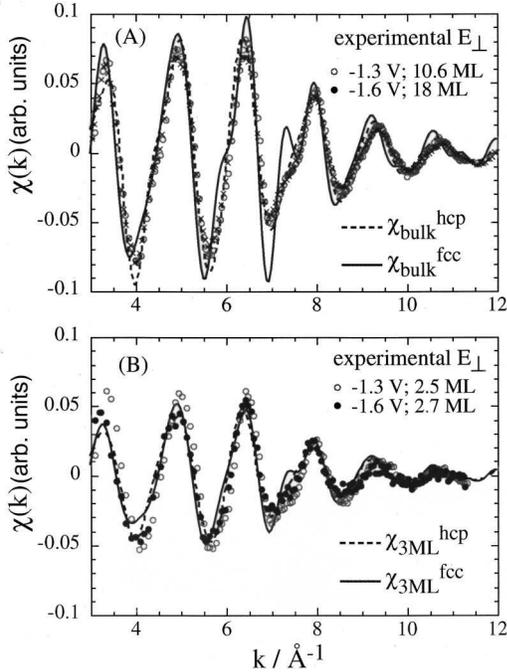
FIG. 9. EXAFS results with out of plane beam polarization. (a) experimental and theoretical  $\chi(k)$  curves for thick layers ( $\geq 10$  ML's); (b) same but for thin layer ( $\leq 3$  ML's). The film thickness and deposition potential are indicated. Data points are experimental and solid or dashed lines are calculated ones. In the case of hcp Co calculation are performed with the  $c$  axis parallel to the beam polarization.
