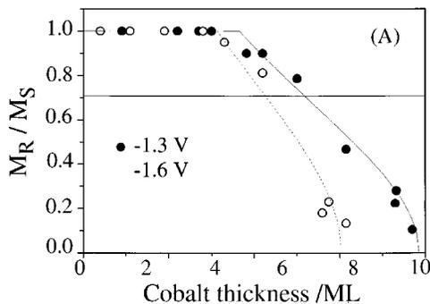
FIG. 4. (a)  $M_R/M_S$  vs  $t$  derived from PMOKE loops of Fig. 3, with  $M_S$  measured at applied field 15 kOe. The solid lines correspond to the plot of Eq. (A7) (see the Appendix, Procedure II). The deposition potential is  $-1.3$  V (bold symbols) and  $-1.6$  V (open symbols).
