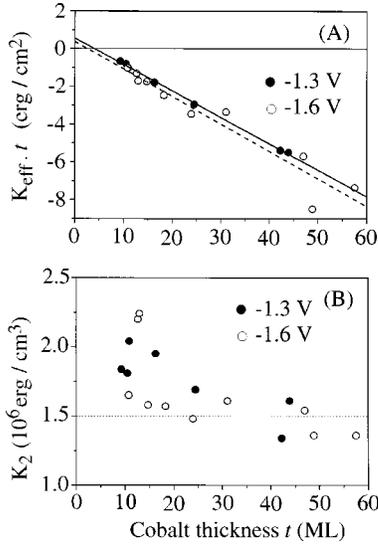
FIG. 11. Parameter determination using Procedure I: (a) Variations of  $K_{\text{eff}} \times t$  vs  $t$ . Straight lines are least-square fits. (b): Variation of  $K_2$  vs  $t$ . The potential of deposition is  $-1.3$  V (solid symbols) and  $-1.6$  V (open symbols).
