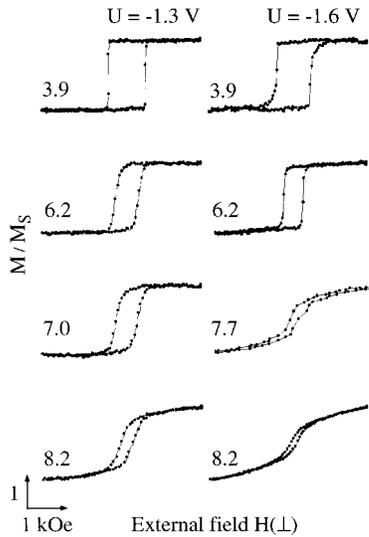
FIG. 3. Normalized PMOKE hysteresis loops obtained with electrodeposited Cu/Co/Au(111) layers. Co deposits were grown at  $-1.3$  V (left) and  $-1.6$  V (right). The figures attached to loops is the Co thickness  $t$  expressed in atomic monolayers (ML's).
