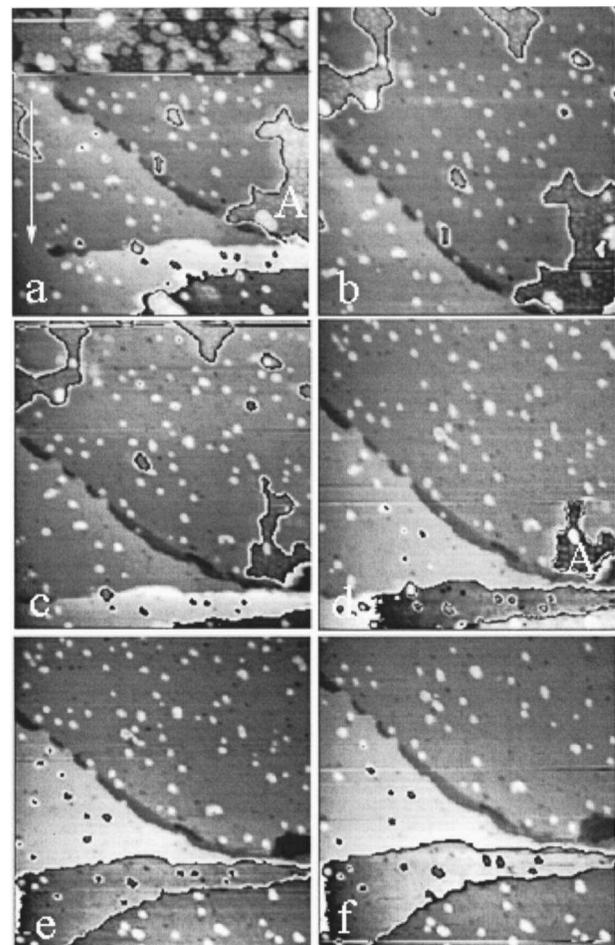
FIG. 8. Six-image STM sequence showing the dissolution of a 3-ML Co layer. The potential was  $U = -1.3$  V in the top of image (a) and was stepped to  $-0.95$  V. Note the nm islands left after stripping. Island (A) is biatomic. The ( $1150 \times 1200$  Å) frames were recorded 50 s apart.
