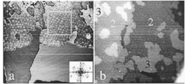
FIG. 7. Sequence of STM images showing the formation of the first three atomic planes of Co at  $U = -1.3$  V. The potential was  $-0.9$  V in the lower half of image (a). The ( $1000 \times 900$  Å) frames were recorded 50 s apart. A Moiré pattern is resolved on each layer; the 2D FFT spectrum in (a) corresponds to the region inside the square box.
