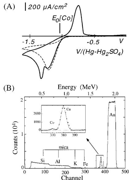
FIG. 2. (a) Cyclic voltammograms of Au(111) in a 1 mM CoSO<sub>4</sub> solution (solid line) and supporting electrolyte (dashed line). Scan rate: 50 mV/s. Supporting electrolyte: 10 mM K<sub>2</sub>SO<sub>4</sub>+0.1 mM KCl+1 mM H<sub>2</sub>SO<sub>4</sub>. (b) Typical RBS spectrum for a Cu/Co/Au(111) trilayer on mica. Elements are indicated in the figure.
