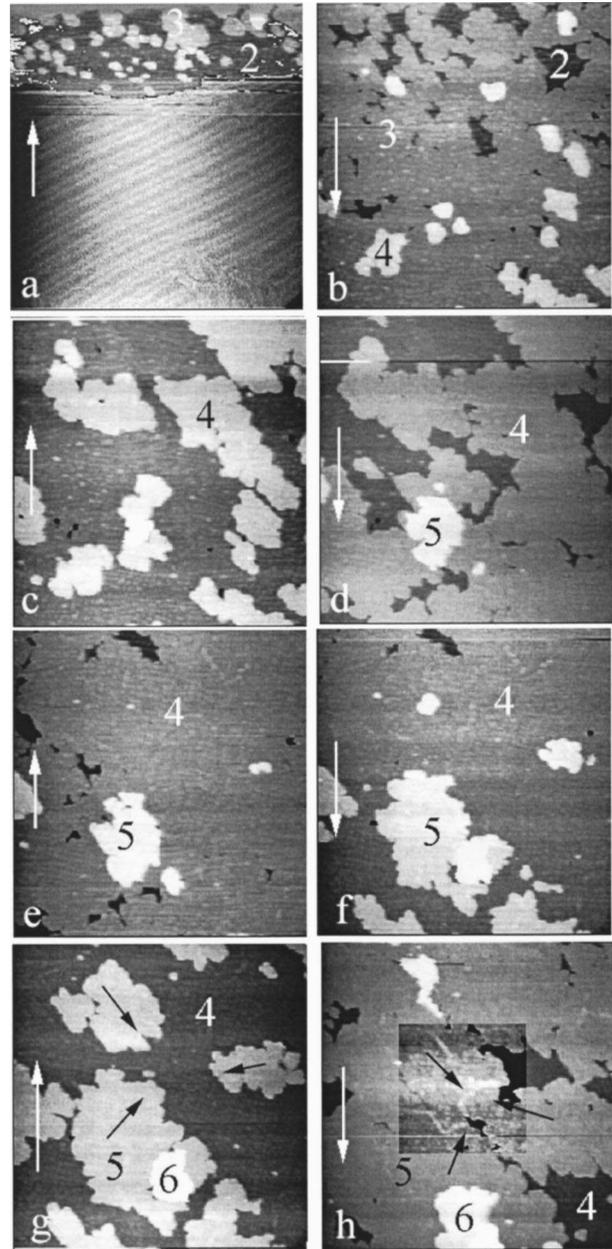
FIG. 5. Sequence of STM images showing 2D growth of Co on Au(111). The deposition potential was  $-1.3$  V. In (a), bottom,  $U = -0.9$  V. The  $(1250 \times 1320 \text{ \AA})$  frames were recorded 50 s apart. Vertical arrows give the direction of slow tip scanning. Figures  $N$  inside images are the local number of Co atomic monolayers. Note the smoothness of the layer. The contrast was enhanced in image (h) to show structural defects in the square box.
